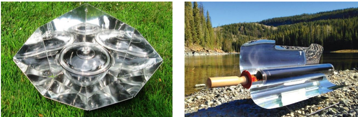
Figure 1.4 The HotPot Solar Cooker (left)[33][34] and the GoSun Stove (right) are examples of small solar cookstoves. Sunlight is reflected and concentrated on a dark inner container that is housed within an optically transparent outer layer. The arrangement creates an enhanced greenhouse effect that can achieve temperatures exceeding 200 °C. The vacuum insulated GoSun Stove can reach temperatures approaching 300 °C.
