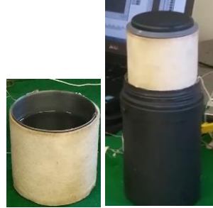
Figure 1.7 Third design iteration of the UCI Stored Thermal Energy Cookstove.
