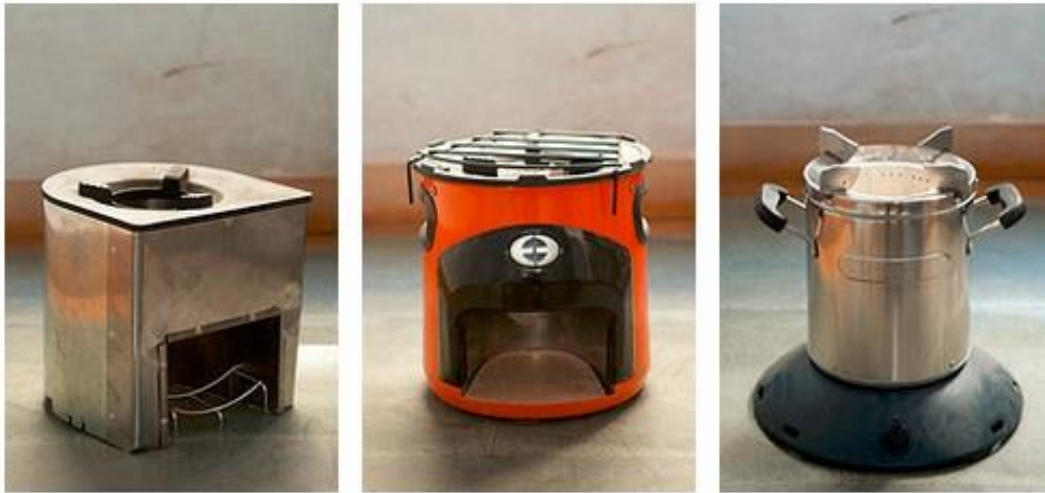
Figure 1.3 Examples of more efficient biofuel burning cookstoves. Efficiency is improved by constricting the air inlet to the combustion zone which leads to a higher velocity draft, improving oxygen supply and increasing combustion efficiency [32].
