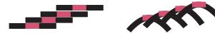
Figure 3: Rendered as disks normal to the viewing direction (downwards), points near each other can form an occluding sequence and appear all black. When rendered as paraboloids (right), like the tapering used in [EBRI09], this is much less likely.
