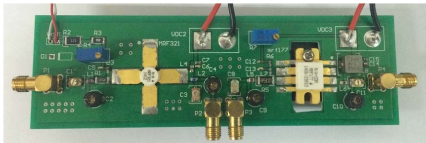
Figure 19 Photograph of one of the MOSFET RF power amplifiers developed for 7 T small animal imaging system
