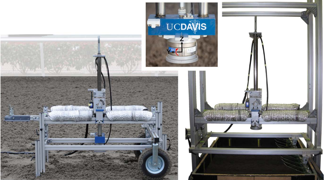
Figure 1. TTD shown on portable frame (left) and laboratory frame (right). The portable frame was leveled and fixed to the ground using 3 adjustable legs. The Z-axis (center) is parallel to the linear shafts (positive up), the X-axis is forward-backward (positive into page), and the Y-axis is lateral (positive left). doi:10.1371/journal.pone.0050534.g001
