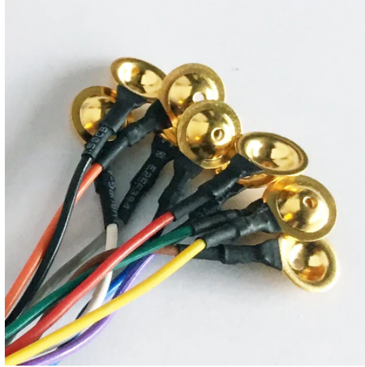
Figure 2.1: Gold-plated cup electrodes used for capturing EMG.
