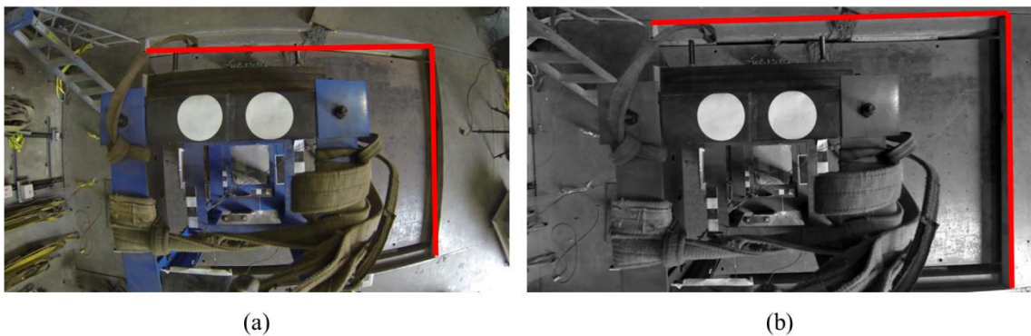
Figure 4.7 Example frames from top-view GOPRO: (a) distorted, color frame, and (b) undistorted, uncolored frame.
