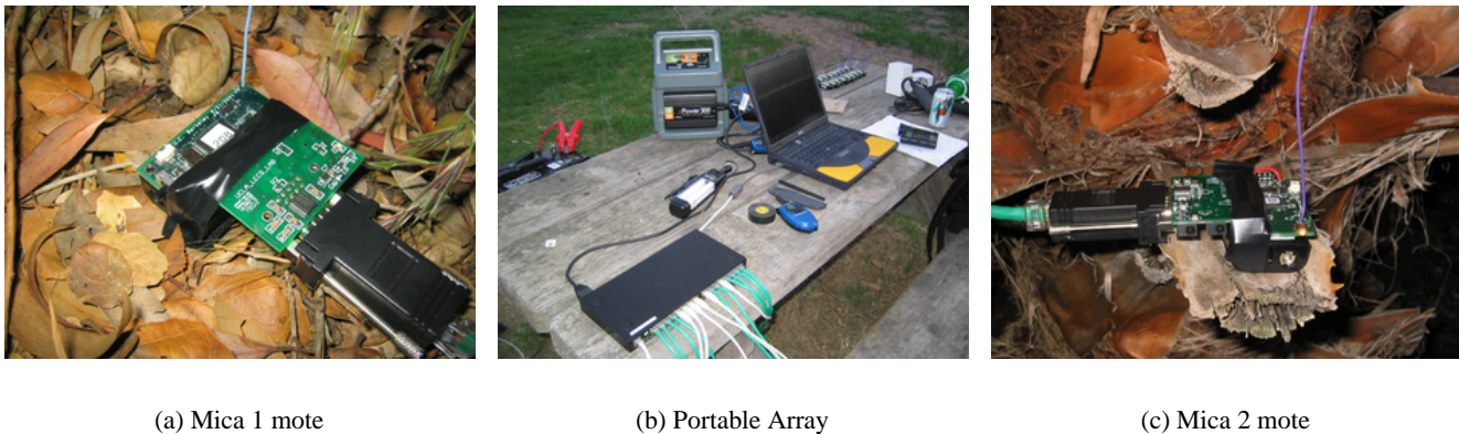
Fig. 1. SCALE hardware. The portable array is composed of a laptop PC attached to a serial multiplexer. Several UTP cables run from the multiplexer to the deployment locations where a mote is attached at the end.
