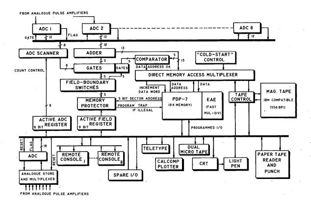
Fig. 1. Block diagram of the PDP-7 data acquisition system.
