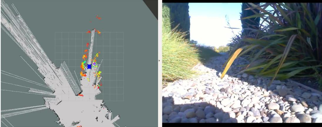
Rover continues along river stones, with wheel slip causing the odometry to drift.
