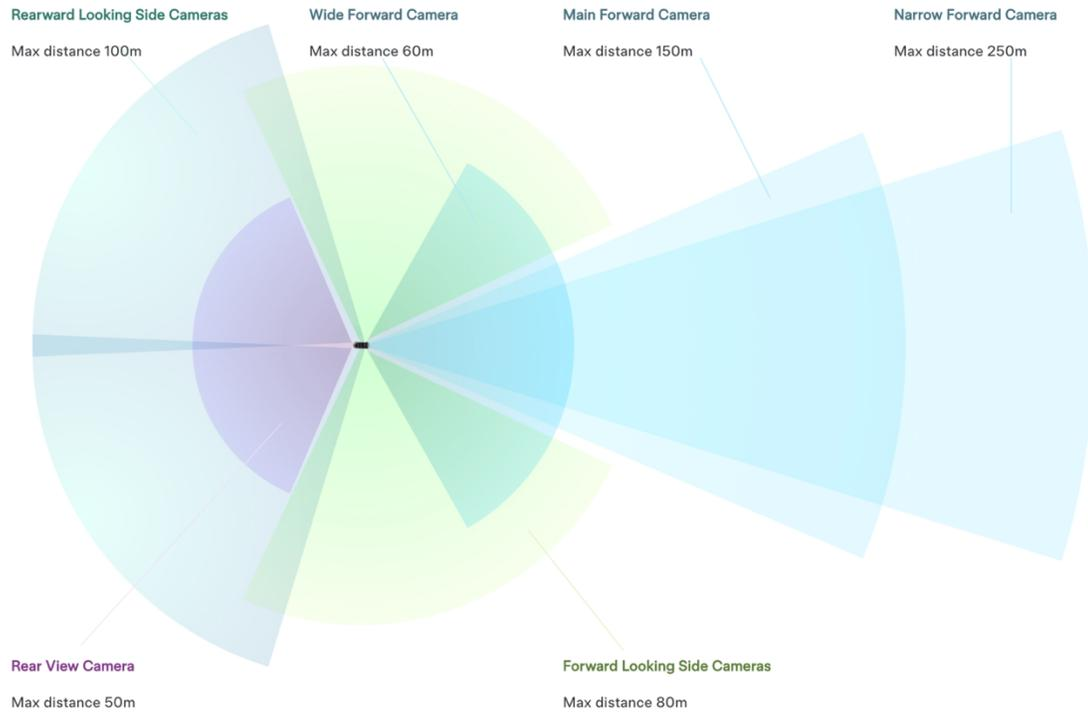
Figure 2.12 Example sensor configuration of on-road autonomous vehicles [29]
