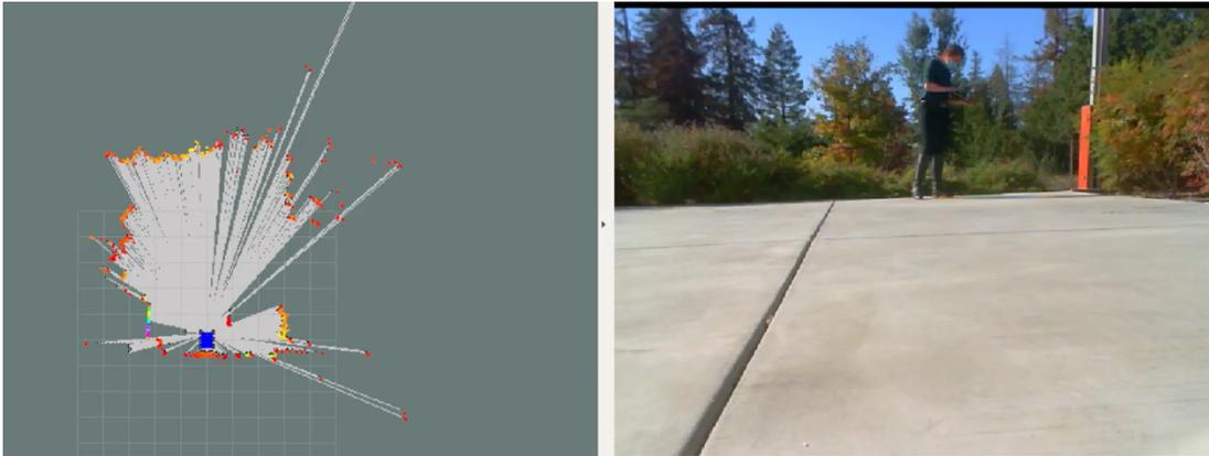
In a new environment, the initial frame of the map is the first frame from the sensors.
