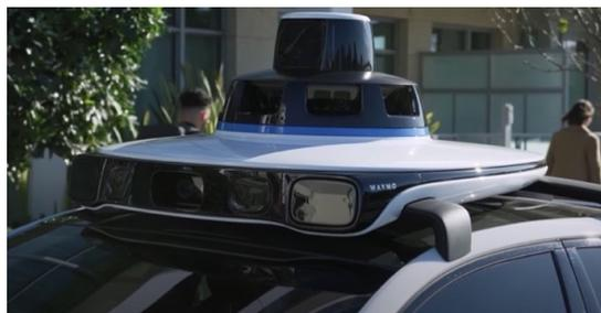
Figure 4.9 Multi camera panoramic array on Waymo self-driving car [54]
