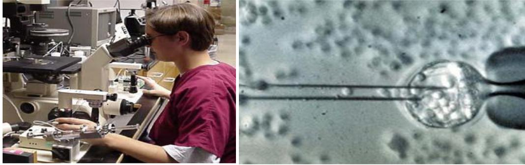
Figure 1.1 Manual operation of gene delivery microinjection into living cells.
