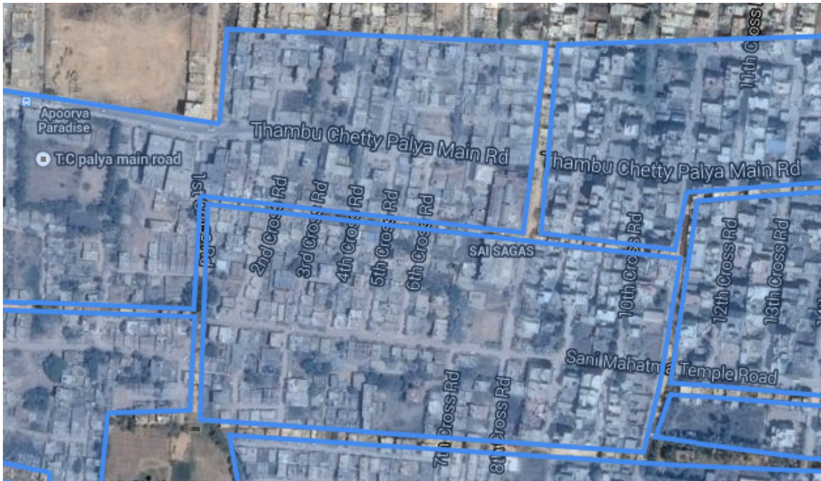
Valve areas from Subdivision E3, Bangalore Water Supply and Sewerage Board (BWSSB). Boundary data provided by NextDrop.
