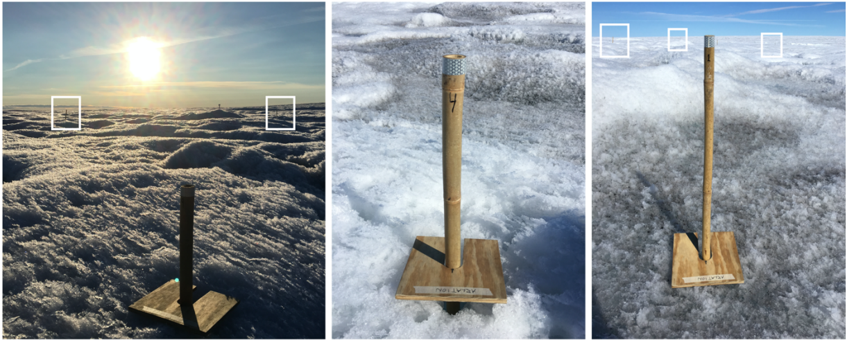
Figure S4-13. A network of twelve bamboo ablation stakes were randomly distributed across an \sim 0.5 \text{ km}^2 area within the study catchment. The distance from the 8x8 inch wooden datum to the top of each stake was measured on a three-hourly schedule from 12:00 on 06 July 2016 to 21:00 on 12 July 2016. The board was oriented true north and 2–4 measurements were made from a line printed on the board to the number printed on top of each stake (visible in images at center and at right) to minimize local ablation rate variability. These distances are converted to cumulative surface lowering for comparison with simulated melt rates. Bright, white ice (center image) contrasts with dark ice (right image). White boxes show stake locations faintly visible in image background.
