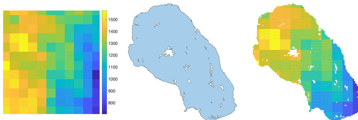
Figure S4-7. Example of processing stream applied to RACMO2.3 climate model output used in this study. (a) The native climate model output is provided at \sim 7.5 km grid spacing. (b) The catchment boundary for 2015 shown here contains internal areas drained by crevasse fields. The native climate model grid is projected onto the National Snow and Ice Data Center Equal-Area Scalable Earth (EASE) and the climate model data is resampled at 100 m horizontal grid spacing using Delaunay triangulation and nearest neighbor interpolation. (c) These 100 m gridded values are then intersected with the lower, upper, and best guess catchment boundaries and converted to volumetric quantities using the catchment-scale area weighted average of the 100 m grid cells at right.
