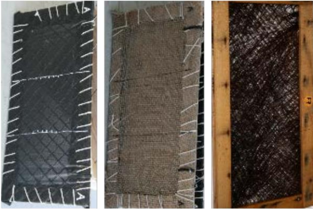
Figure 4.1: Different egg frame materials (right to left: palm tree fiber, burlap, and garden fabric).
