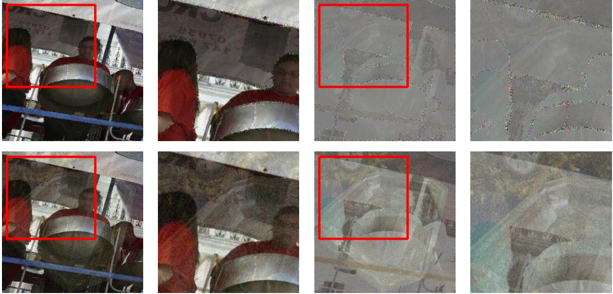
Figure 5.2: Visualization of experimental results. First row: PL (ours); Second row: L_2 -distance. From left to right: adversarial image, a zoomed patch, the corresponding noise, zoomed noise patch. Our method can effectively reduce the ghosting artifacts within the red box.
