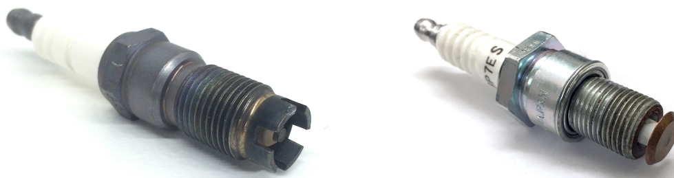
Figure 4.3: Diagrams of spark plugs used in this investigation. The geometry on the left is the same as that used by Sjöberg et al. (2014) and Sevik et al. (2016) in internal combustion engine experiments, while the geometry on the right represents an attempt to achieve multi-point ignition.
