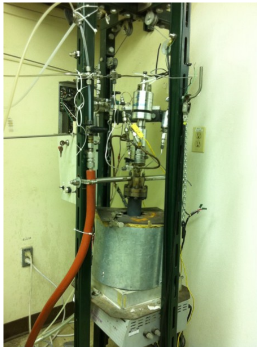
Figure 2.4 A schematic diagram and photo of the stirred batch reactor (1. Magnetic agitator 2. Thermocouple 3. Electrical furnace 4. Inconel reactor 5. Impeller coupled with agitator)
