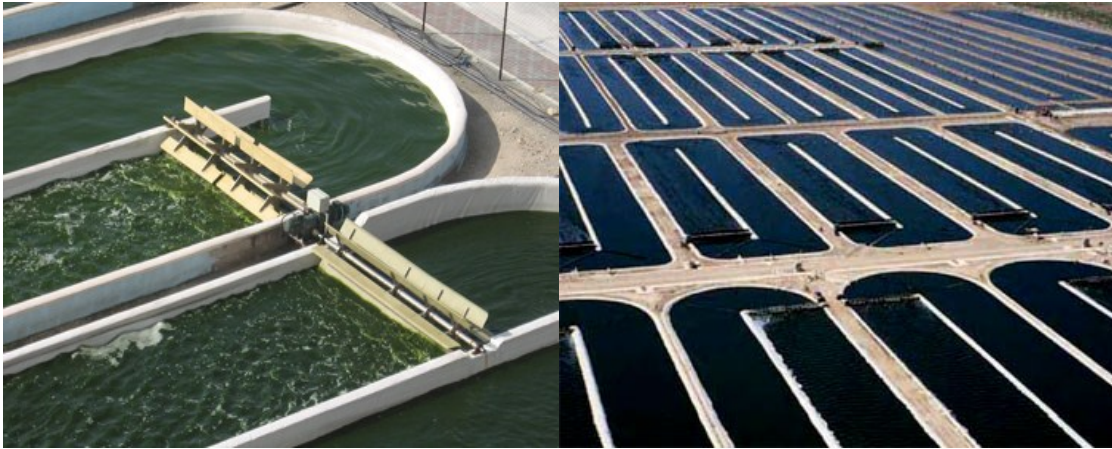
Figure 1.1 Open ponds system, pictures courtesy of Seambiotic, Ltd. (left) and pictures courtesy of energybiosciencesinstitute.org (right)
