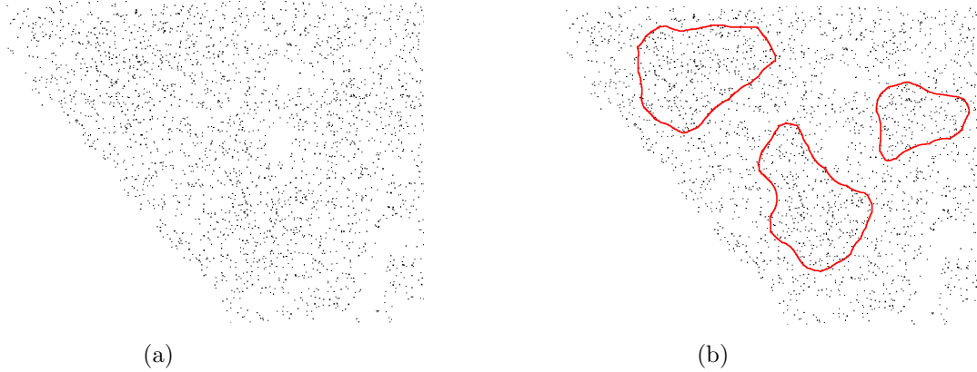
Figure 2.8: A 2500 event sample of the density function from Figure 2.7 is shown in (a). The contour of the segmented dense region is shown in (b). The choice of parameters is: \mu = 0.11 , timestep is 11.0 with the 3-step adaptive resolution. The data points in this figure are manually enhanced for the purpose of more clear display of the image.
