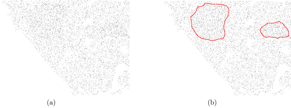
Figure 2.6: An 8000 event sample of the density function from Figure 2.4 is shown in (a). The contour of the segmented dense region is shown in (b). The choice of parameters is: \mu = 0.092 , time step is 8.0 with the 2-step adaptive resolution. The data points in this figure are manually enhanced for the purpose of more clear display of the image.
