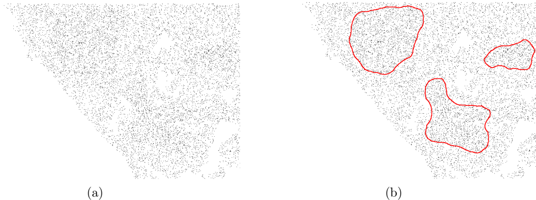
Figure 2.9: A 10000 event sample of the density function from Figure 2.7 is shown in (a). The contour of the segmented dense region is shown in (b). The choice of parameters is: \mu = 0.075 , timestep is 7.5 with the 2-step adaptive resolution. The data points in this figure are manually enhanced for the purpose of more clear display of the image.
