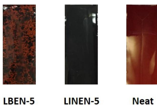
Figure 6.7 Image of LBEN–5, LINEN–5 and neat network. Neat network represents the epoxy network prepared from GEDHEO–NOVO and DETA, with no addition of organosolv lignin.
