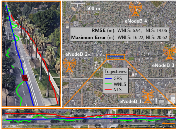
Fig. 7. Experimental results for positioning with LTE SSS signals in downtown Riverside, California, using: (i) WNLS estimator whose weights were calculated to (12) and (ii) NLS estimator. The position errors are calculated with respect to the GPS solution. Image: Google Earth.
