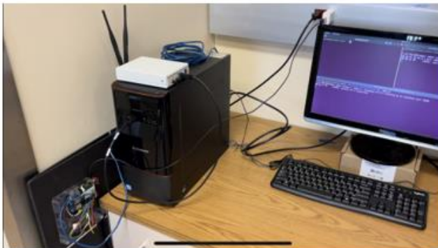
Figure 3. Implemented setup of the USRP modules as a) broadcast and b) receive.
