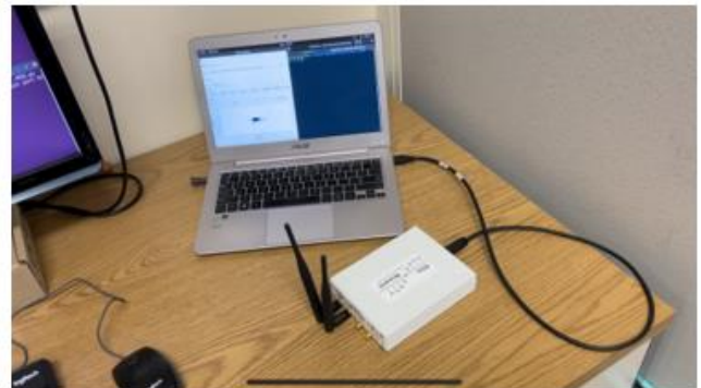
Figure 3. Implemented setup of the USRP modules as a) broadcast and b) receive.
