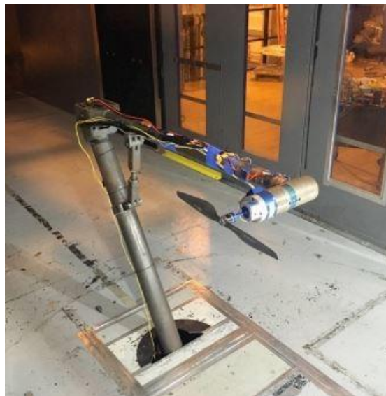
Figure 3.6: Hover test for the SUI isolated rotor in 7- by 10-Foot Wind Tunnel [46]
