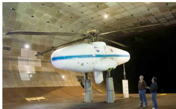
Figure 2.15: UH-60A airloads rotor in the 40- by 80-Foot Wind Tunnel at Ames Research Center (ARC) [35]
