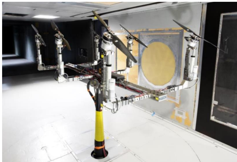
Figure 1.2: MTB in the 7- by 10-Foot Wind Tunnel at Ames Research Center [4]
