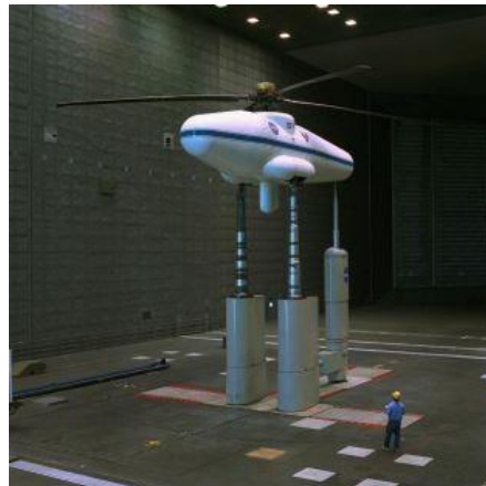
Figure 3.2: UH-60A rotor system at the National Full-Scale Aerodynamics Complex wind tunnel [44]
