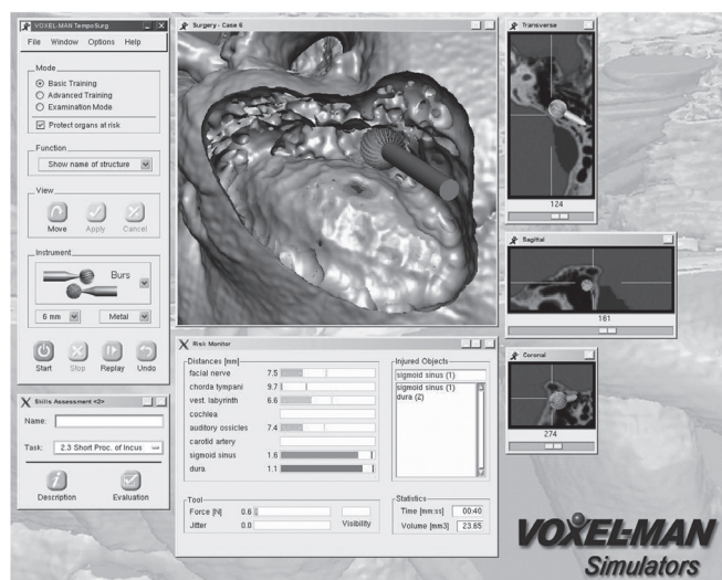
Fig. 2. The VOXEL MAN TempoSurg® user interface. In this case, the sigmoid sinus (blue) and the dura (brown) are injured. The surgeon is on the way to the antrum which is not opened. This is the mode for beginners. The risk monitor, which shows the distance to vital structures, can be seen at the bottom. A 3-D-navigation is displayed on the right side. An interactive menu to choose the level, the view and the instrument is on the left side.
