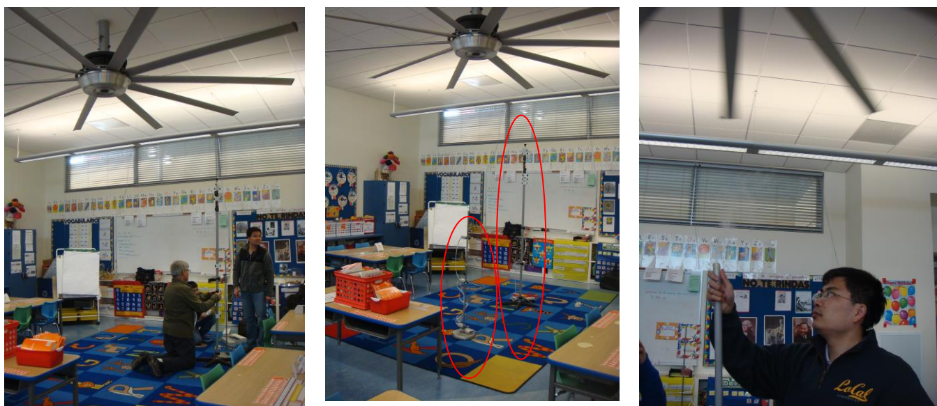
Figure 63 Airspeed measurement and flow visualization in classroom 1 in an open space
