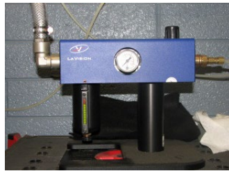
Figure 3-8: LaVision Olive oil seeder.
