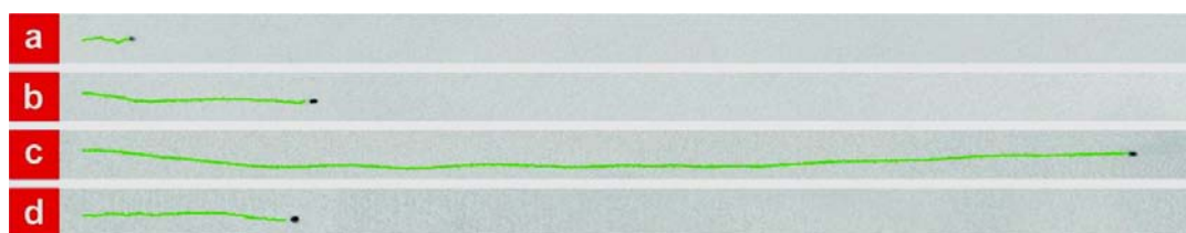
Figure 1.2.2 Nanomotor racing: Optical images, superimposed with track lines, illustrating the speed of magnetically-guided Au/Ni/Au/Pt (a, d) and Au/Ni/Au/Pt-CNT (b, c) nanomotors, using 2.5% hydrogen peroxide, with (c, d) and without (a, b) 0.15% hydrazine. (Reprinted with permission from ref. 44. Copyright 2008 American Chemical Society.)
