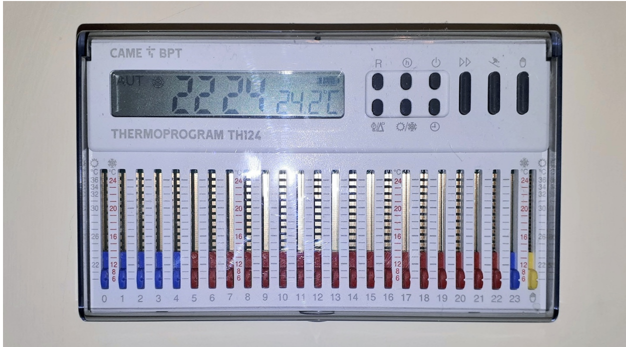
2 Figure 6: Example of a programmable thermostat where the hourly temperatures setpoints are chosen using sliders.
