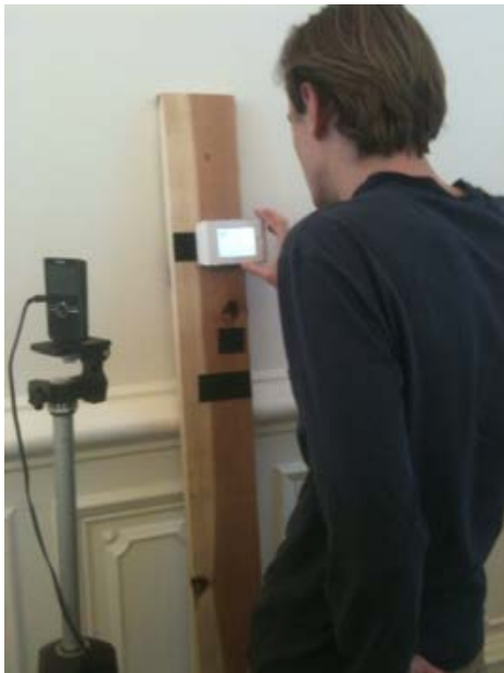
Figure 1. Laboratory set-up for measuring the usability of a thermostat.
