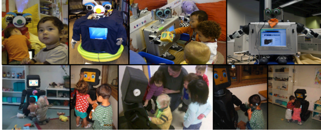
Figure 2.1. Top row: RUBI progression: from left to right RUBI-1, RUBI-2, RUBI-3 & RUBI-4. RUBI-1 and 2 were remotely operated. RUBI-3 was the first fully autonomous design. Bottom row: RUBI-5 playing with kids at ECEC classroom 2A.
