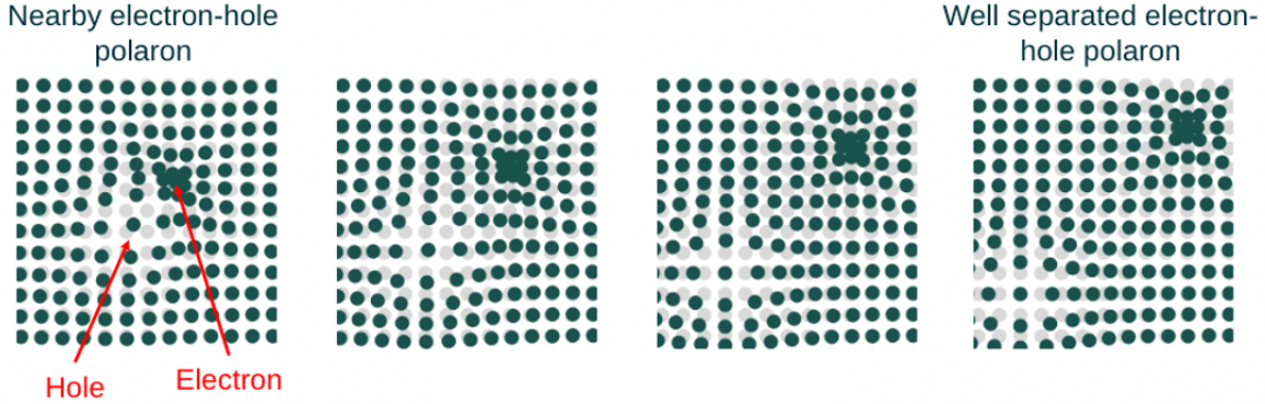
Figure 5.7: Depiction of the polaron cloud interference for nearby electron-, hole-polarons (left most panel) and distant electron-, hole-polarons, (rightmost panel). Grey dots are the pristine lattice while teal dots show how the lattice distorts in the presence of the electron and hole.
