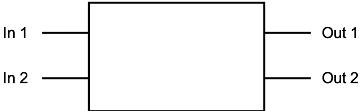
Figure 3.5: A block diagram of a switch cell in which there are two inputs and two outputs.
