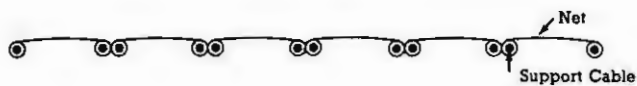
Figure 5. Each net edge is looped around the support cable and hog-ringed to itself. The outermost net edge is attached to the perimeter ground cable.
