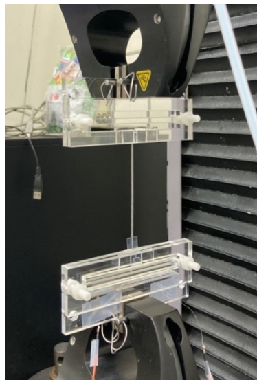
Figure 2.8 Image of e-band clamped by a stretching setup
