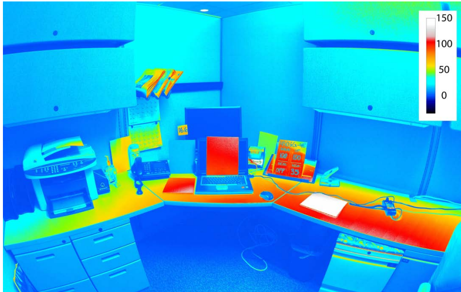
Figure 15: False color image of workstation 35 with overhead lights at 100% and undercabinet light off. Calibration bar is in candelas per meter squared.
