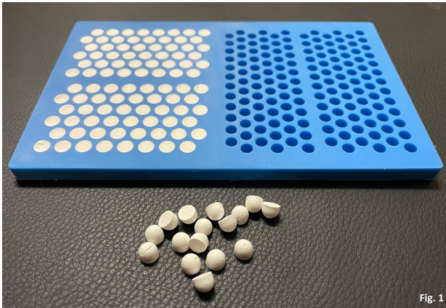
Figure 1. Picture of antibiotic-loaded \text{CaSO}_4 beads showing a 6 mm bead mat with cured \text{CaSO}_4 beads. Harvested beads next to the bead mat show the hemisphere shape of the beads.
