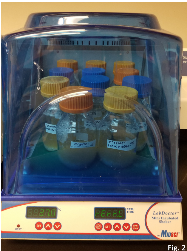
Figure 2. Simulated large joint fluid model setup. The 250 mL Pyrex container contains 70 mL of test fluid with 35 mL of \text{CaSO}_4 beads (totalling 175 beads) added to the fluid. The container sits atop a mixing stand stored in a sterile environment. The metal plate upon which the bottles rest is set on low shake to gently mix the fluid.
