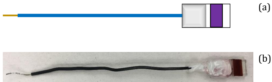
Figure 3.2: (a) schematic display of fabricated working electrode (b) \text{OsCl}_2 dyed working electrode
