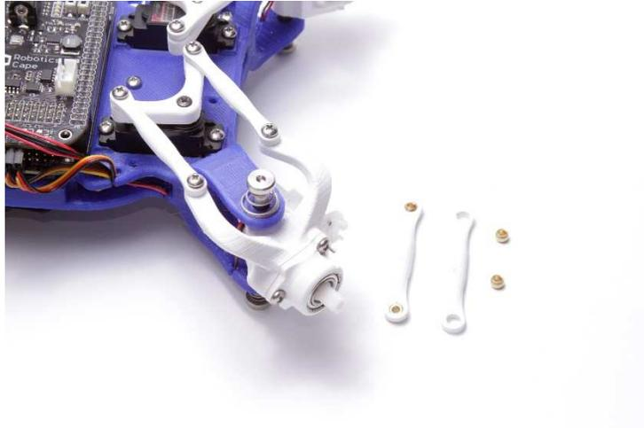
Figure 3.1: Close up of four bar steering mechanism.
