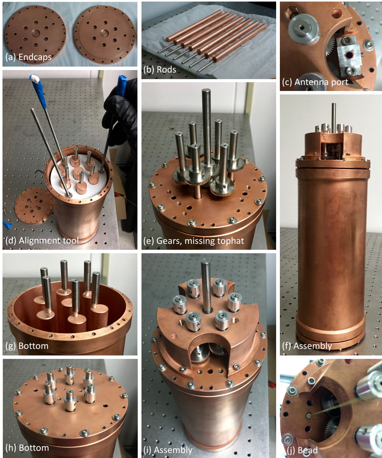
Figure 4.3: Seven-rod cavity photos after copper-plating and re-machining.
