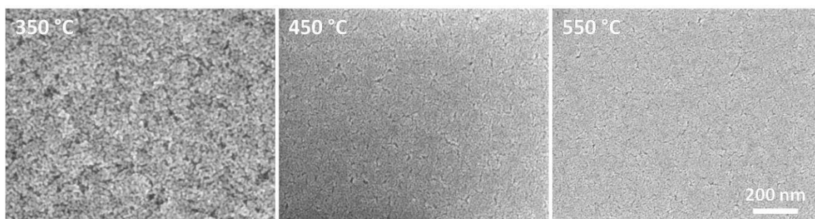
Figure 7. Surface morphology of post-heat treated Sol-Gel prepared double-layer NiO thin films by spin-coating at 3000 rpm. The films were annealed in N_2/O_2 environment at different annealing temperatures (i.e. 350, 450, and 550 °C)
