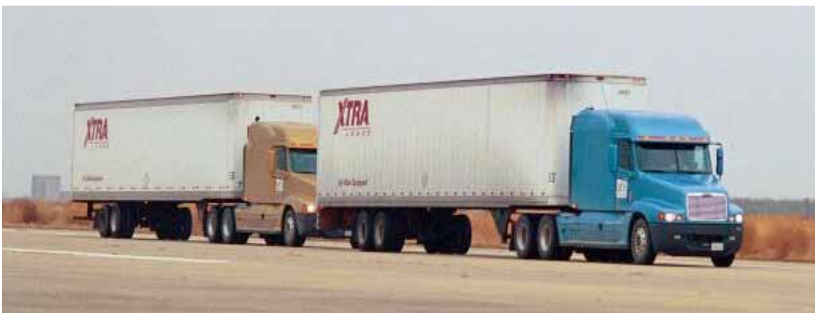
Figure 2. The two Freightliner trucks running southbound at 3-meter spacing, December 4, 2003.
