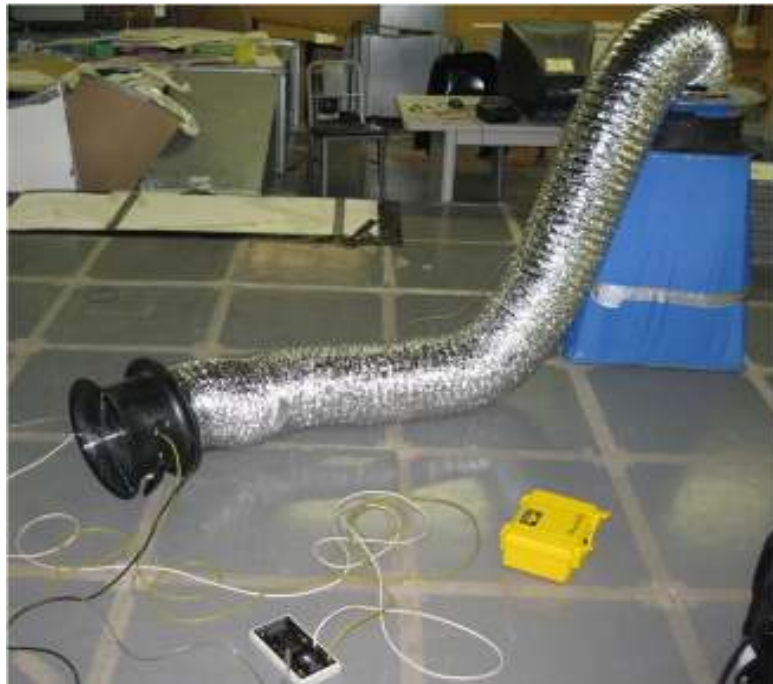
Figure 4-12 Duct blaster configuration
