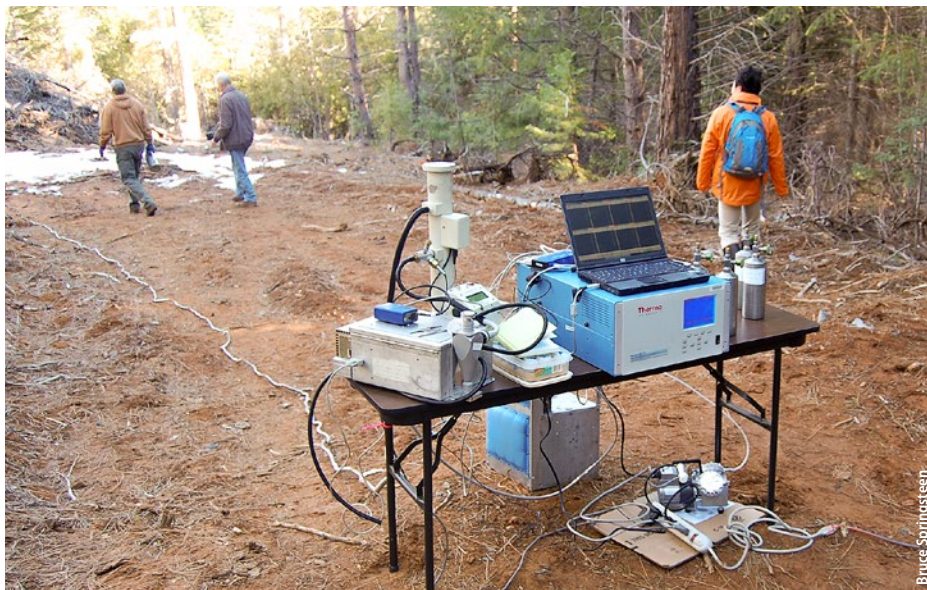
Fig. 2. To sample air emissions from the pile burn, researchers used a 20-foot steel probe at the edge of the pile (top); nitrogen oxides, black carbon and carbon dioxide were measured on site using continuous emissions monitors. Canister samples were collected and sent for offsite analysis for total fine particulate matter, trace hydrocarbons and carbon monoxide.
