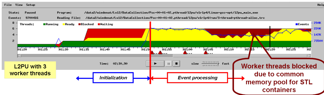
Figure 90. Event processing in three concurrent worker threads. It can be seen that for a substantial fraction of time the worker threads block each other during event processing. This is due to an inefficient memory allocation scheme used in an older version (gcc 2.96) of the C++ Standard Template Library .
