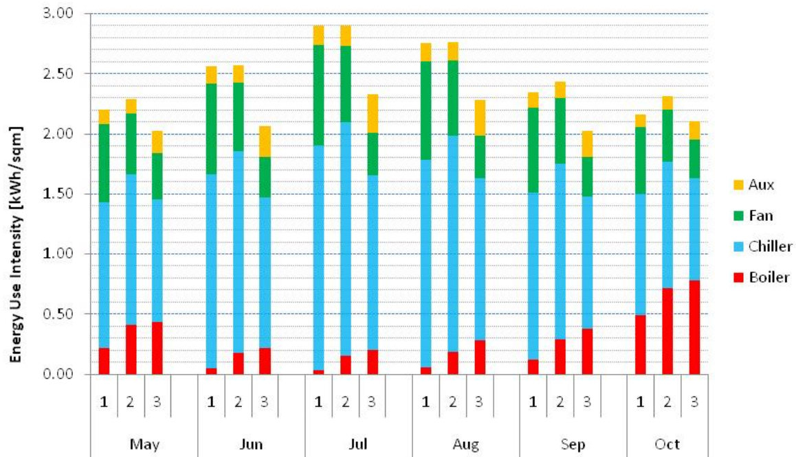
Figure 6: Cooling season HVAC energy consumption for each of the runs described in Table 2.
