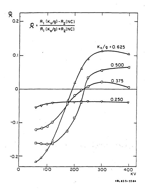
Fig. 2. Variation of the electron induced characteristic x-ray emissions as a function of the accelaration voltage for fixed excitation errors. Normalization is done with respect to a non channelling (NC) symmetric orientation.
