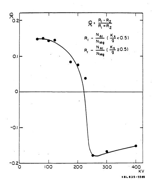
Fig. 1. Variation of the electron induced charateristic x-ray emissions with both orientation and acceleration voltage. Calculations were performed for 15 beams, systematic excitation condition (g = 400).
