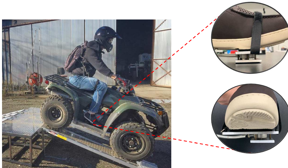
Figure 1.2. Foot brake testing, with button (foot)-loadcell interface: (a) side view, and (b) front view
