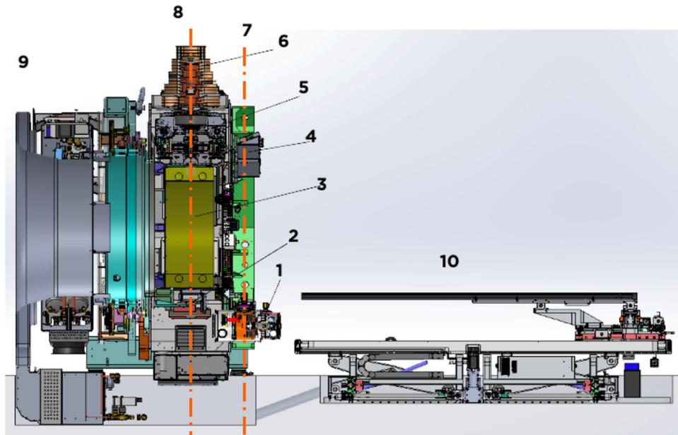
**FIGURE 1** Section view of the RefleXion X1 linac with components: (1) kvCT X-ray tube; (2) MV EPID; (3) PET detectors; (4) kvCT detector; (5) primary collimators; (6) 6MV linac; (7) kvCT plane; (8) MV and PET plane; (9) cooling system; and (10) couch
