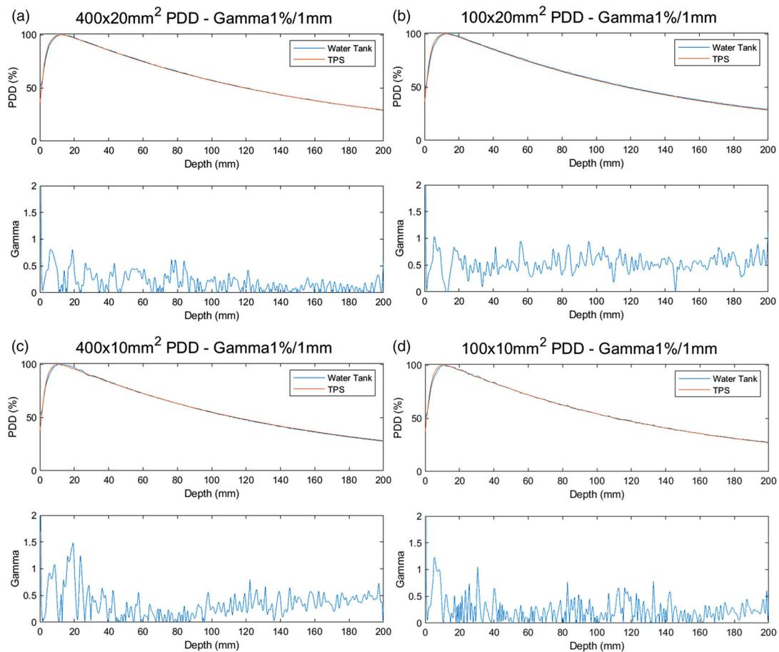
**FIGURE 7** PDD curves of measurement and TPS calculation with 1D gamma analysis for: (a)  $40 \times 2 \text{ cm}^2$  field; (b)  $10 \times 2 \text{ cm}^2$  field; (c)  $40 \times 1 \text{ cm}^2$  field; and (d)  $10 \times 1 \text{ cm}^2$  field
