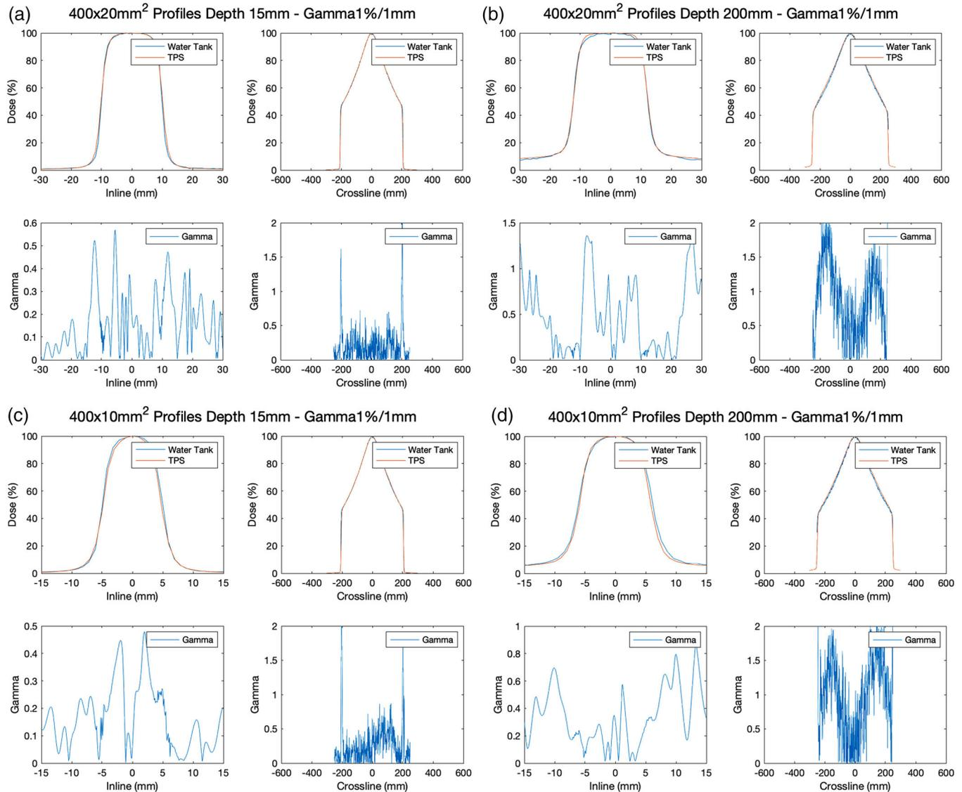
**FIGURE 9** Measured and TPS calculated longitudinal (inline) profiles of: (a)  $40 \times 2 \text{ cm}^2$  field at 1.5 cm depth; (b)  $40 \times 2 \text{ cm}^2$  field at 20 cm depth; (c)  $40 \times 1 \text{ cm}^2$  field at 1.5 cm depth; and (d)  $40 \times 1 \text{ cm}^2$  field at 20 cm depth
