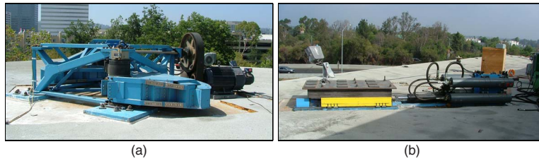
Figure 5. Field shakers: (a) eccentric mass shaker (EMS) and (b) linear mass shaker (LMS).
