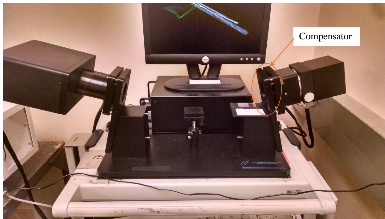
Figure F-2 Sample stage, light source and compensator of ellipsometer .
