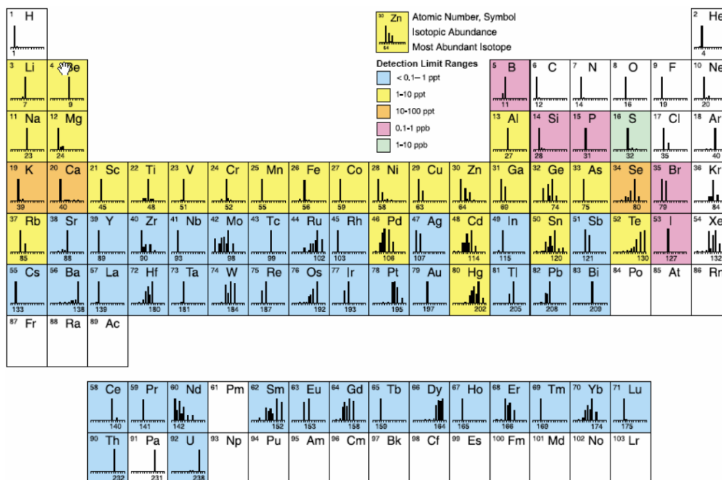
Figure 2-13. Periodic table of elements measured by ICP-MS along with their corresponding detection limit ranges for ELAN series mass spectrometers. All of the elements studied in this work have limit ranges between 0.1-10 parts per trillion. (Image courtesy of PerkinElmer, Inc.)
