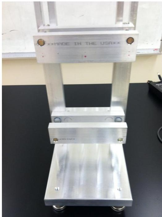
**Figure 29** Photo of fabricated percussion test fixture.
