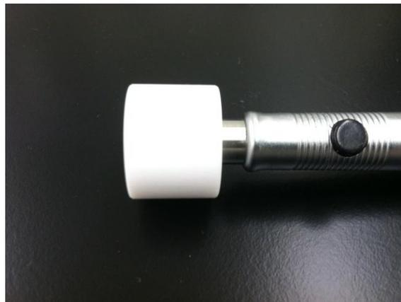
**Figure 30** Photo of the one inch diameter Teflon nozzle.
