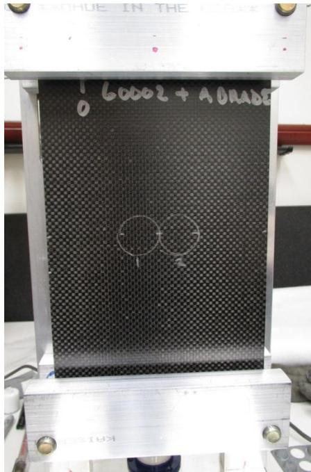
Figure 75 Control NDI panel attached to the aluminum test fixture.
