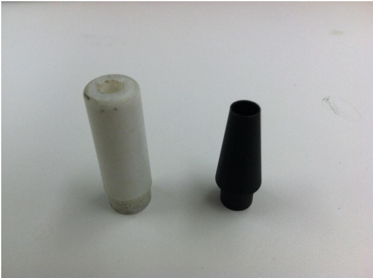
**Figure 25** Illustration of black plastic and white Teflon nozzles used to direct the percussion rod onto the test specimen surface.
