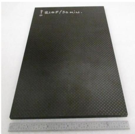
**Figure 73.** Illustration of a 6.35 mm (0.25 in.) thick secondary bonded composite panel fabricated for bond strength variation study.
