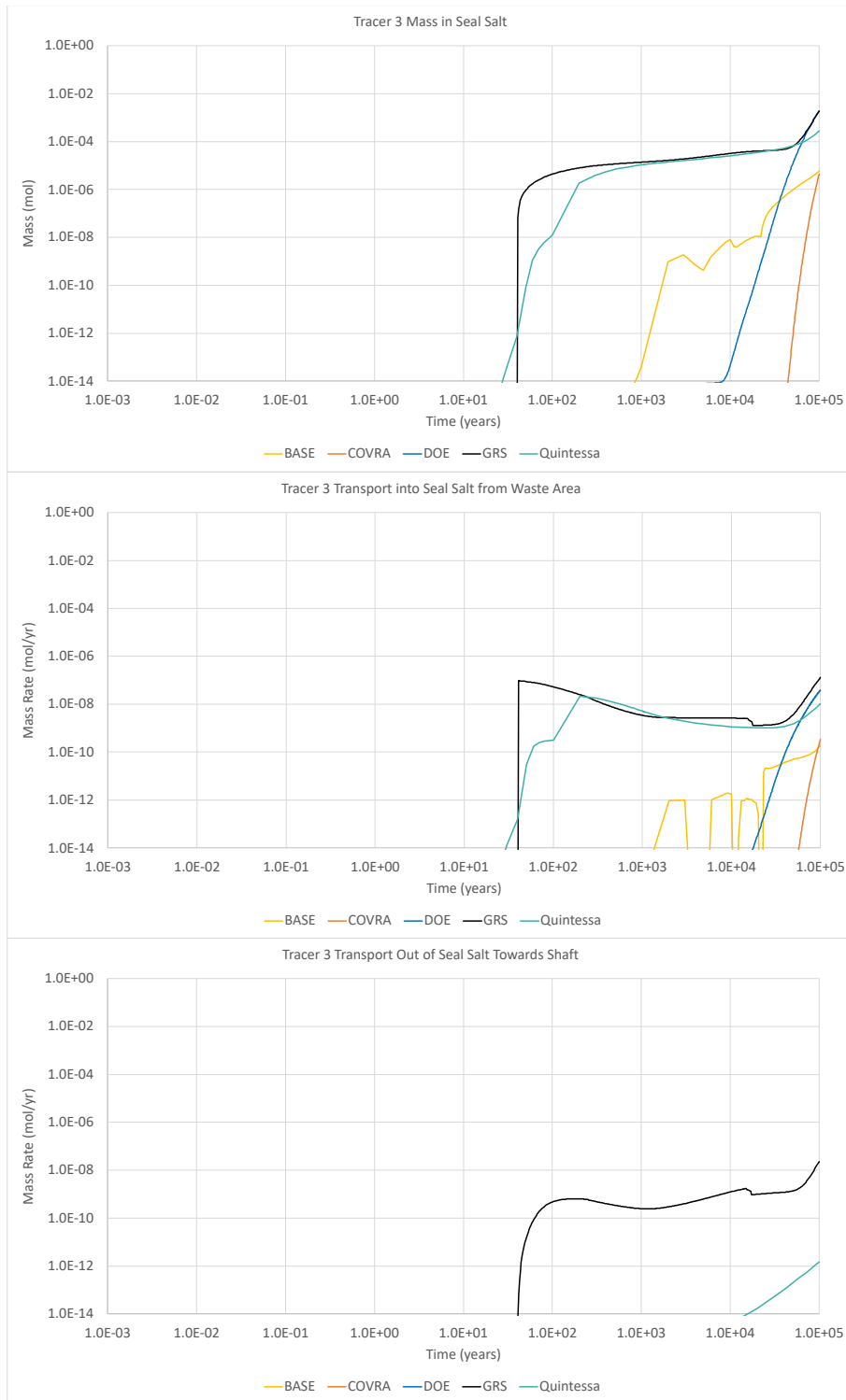
Figure 5-10 Tracer 3 transport quantities the salt in the repository seal. Top: Tracer 3 mass. Centre: Tracer 3 transport between the salt and drifts connecting to the waste area. Bottom: Tracer 3 transport between the salt and drifts connecting to the shaft. Positive is defined as transport out of the repository and towards the shaft.
